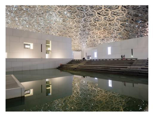
These stars are repeated in various sizes and angles to form eight different layers. The four outer layers are made of stainless steel and the four inner layers are made of aluminium.
